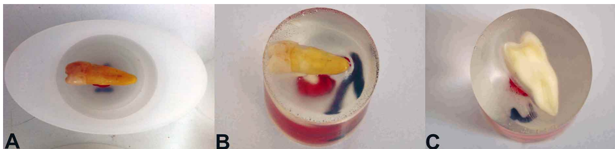
Fig. 1. Preparation of the specimens. A) tooth positioned within the silicon mold and embedded in epoxy resin. B) Polymerized resin cylinder released from mold and C) Upper view of an abraded and polished dentin surface.
